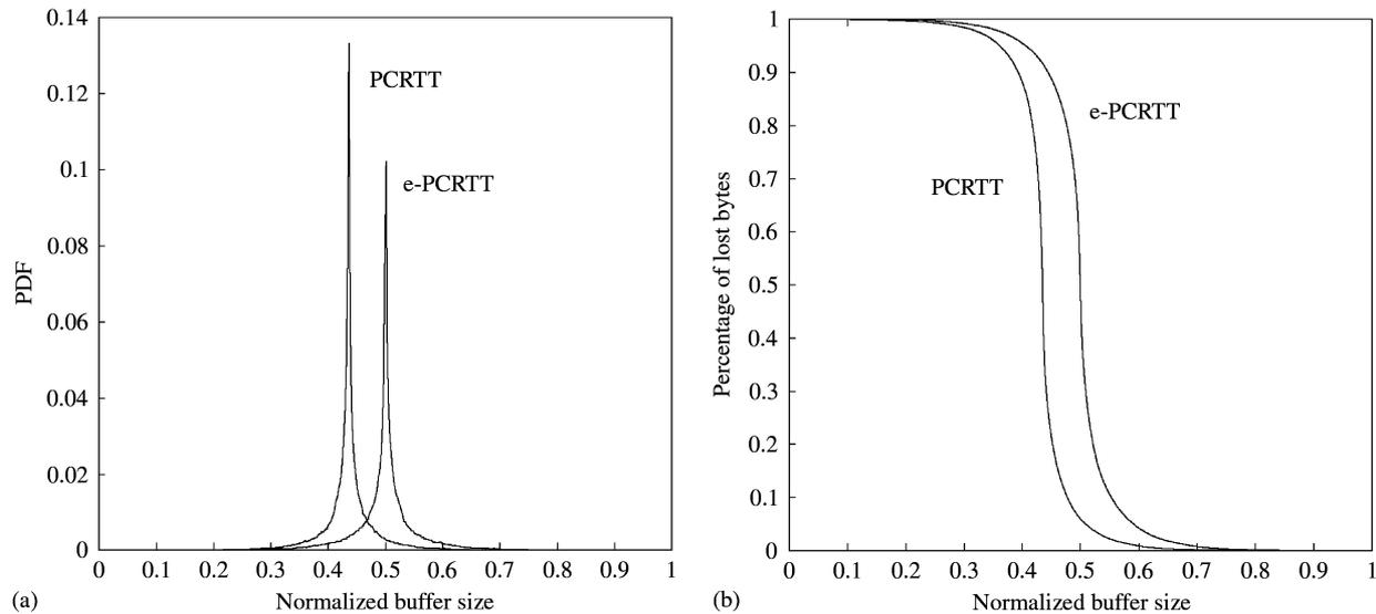
**Figure 6.** Buffer utilization for E.T (100) video trace. (a) Probability Density Function of the buffer content; (b) Percentage of loss bytes.
