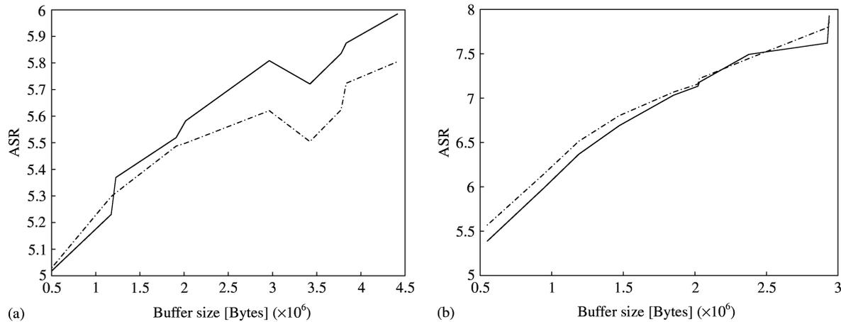
**Figure 10.** Average-to-Std, Ratio (ASR) as function of the buffer size. (a) E.T (100); (b) Rookie of the Year (90). — PCRTT; - - - e-PCRTT.
