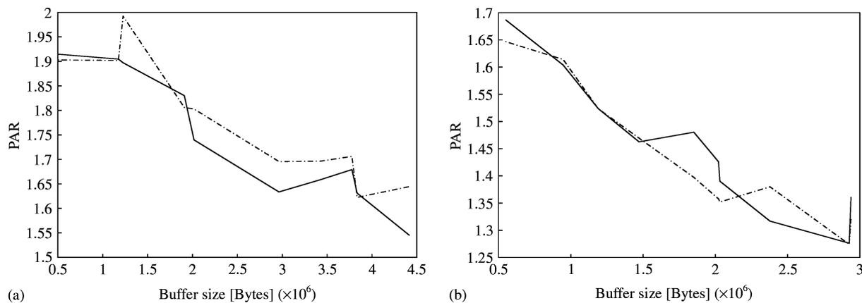
**Figure 9.** Peak-to-Average Ratio (PAR) as function of the buffer size. (a) E.T. (100); (b) Rookie of the Year (90). — PCRTT; ---- e-PCRTT.
