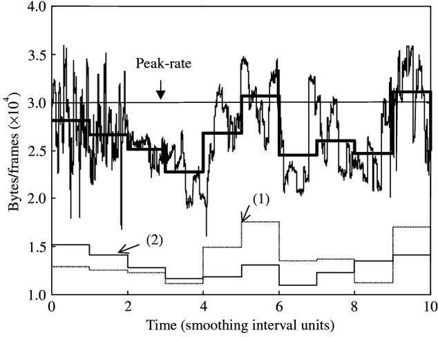
**Figure 11.** An example multiplexing two video streams into a CBR channel before and after bandwidth smoothing. — Combined smoothed streams; jagged line=combined unsmoothed stream.
