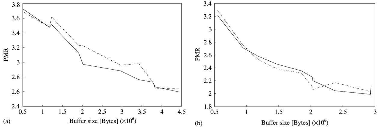
**Figure 8.** Peak-to-Min ratio (PMR) as function of the buffer size. (a) E.T. (100); (b) Rookie of the Year (90). — PCRTT; ---- e-PCRTT.
