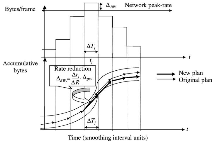
**Figure 12.** The management process of bandwidth rate reduction at the  $j$ 'th interval.
