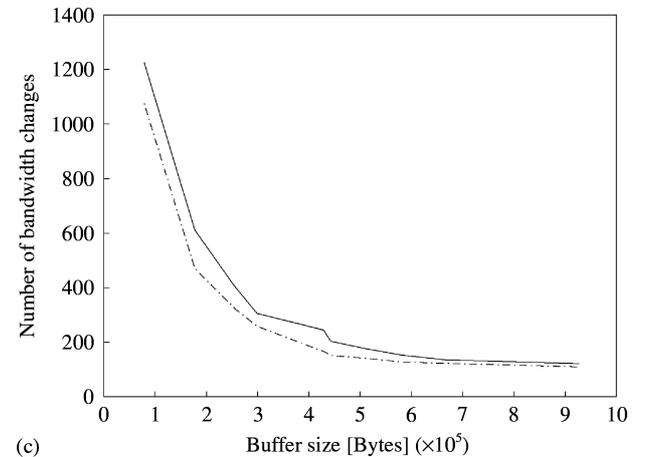
**Figure 5.** Minimum number of bandwidth changes as a function of the buffer size for three video streams. (a) E.T (100); (b) Rookie of the year (90); (c) Seminar-2 (90). — PCRTT; - - - e-PCRTT.
