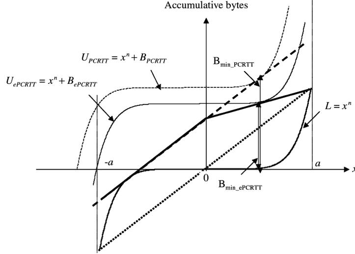
**Figure 3.** Minimum buffer derivation for the analytical function  $x^n$ , for the two algorithms PCRTT and e-PCRTT.
