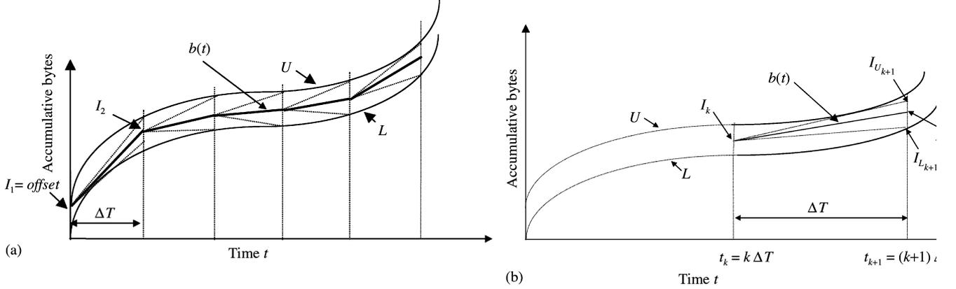
**Figure 1.** The Enhanced PCRTT Algorithm. (a) The construction process; (b) Parameter definitions.
